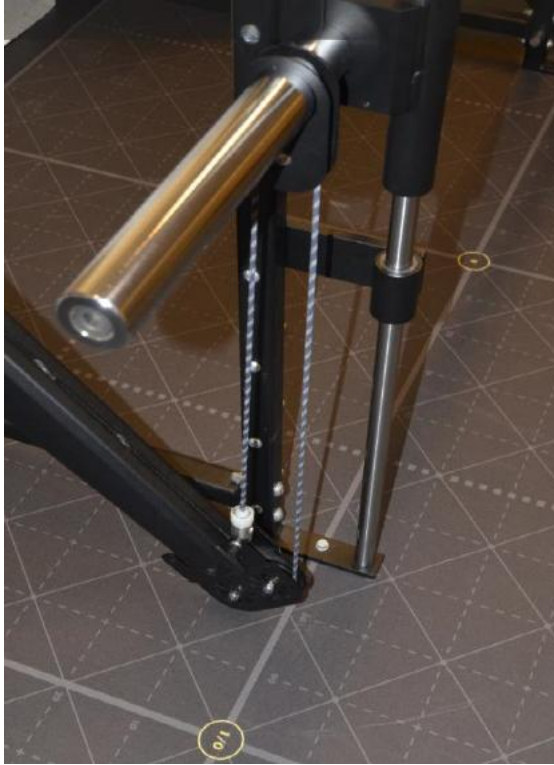
Pulley (Gear 2) setup on a Syncro Smith. On a single machine a pulley is hooked up to the handle.
